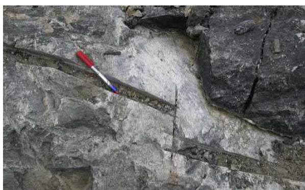
Figure 2- Channel sample cut by pneumatic drill machine for exploration of platinum-group elements at open pit bench face, Boula-Nausahi chromite mine, Orissa, India.
