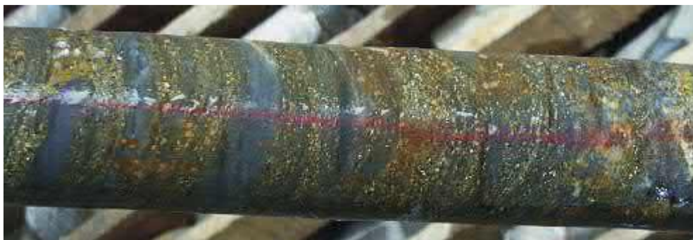
Figure 8- Standard drill core showing stratiform sphalerite and galena in calc-silicate host rock with the red pencil line marked for splitting into two near-identical halves at Rajpura-Dariba Mine, India.
